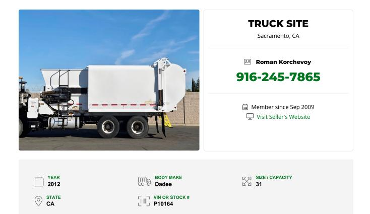
2012 Dadee MFG Scorpion Automated Side Loader Body & Arm, 21 Cubic Yard Body, Packer Performance up to 750 lbs per Cubic Yard & 14-17 Second Auto-Pack Cycle, PAPP Scorpian Arm (2,000 lb Lift Capacity, Under 8 Second Cycle Time & 98" Reach), Self-Cleaning Packing Mechanism, Joystick Controls, Includes all Cylinders, Brackets, Wiring and Controls, Fits on 184-194" Cab to Axle & 201-220" Wheelbase, Very Clean & Well-Maintained Ex-City Unit
