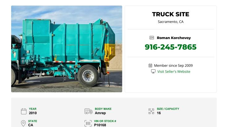
2010 Amrep AMOCASLTPO-14 Automated Side Loader Body, 16 Yard Capacity, Dump Eject, 300-900lb Arm Capacity (109" Arm Reach), Packer Blade, Mounts on 160" Wheelbase and/or 144" Cab to Axle, Well-Maintained Ex-City Unit
